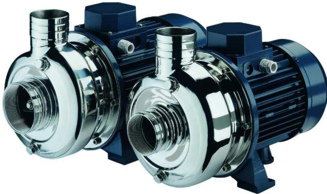
Opened impeller pumps fully made of stainless steel suitable for domestic, agricultural and industrial applications. All parts which are in contact with the pumped liquid are in Aisi 304 stainless steel in order to grant a maximum hygiene and resistance against corrosion. The open impeller allow pumping of clean or relatively dirty water which have solid parts with diameter maximum of 8 mm.
